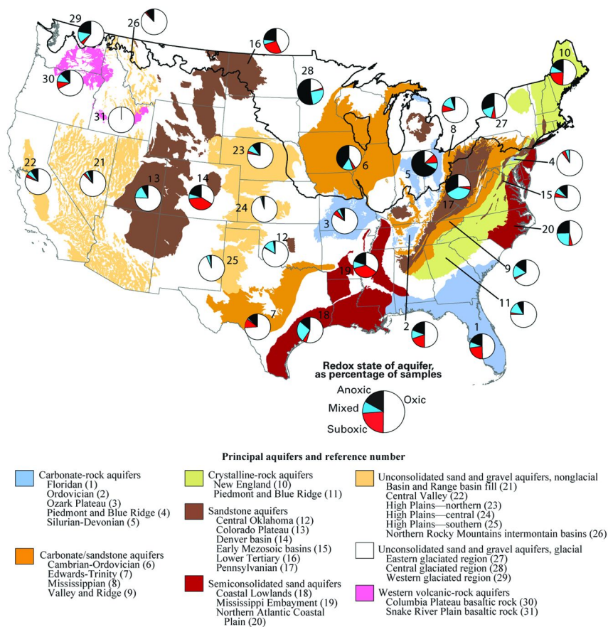
Figure 8. Pie diagrams indicating the percentages of domestic well samples that were oxic, suboxic, anoxic, or diagnostic of mixed redox processes in selected regional aquifers of the United States. (modified from reference (58)) (see color insert)
